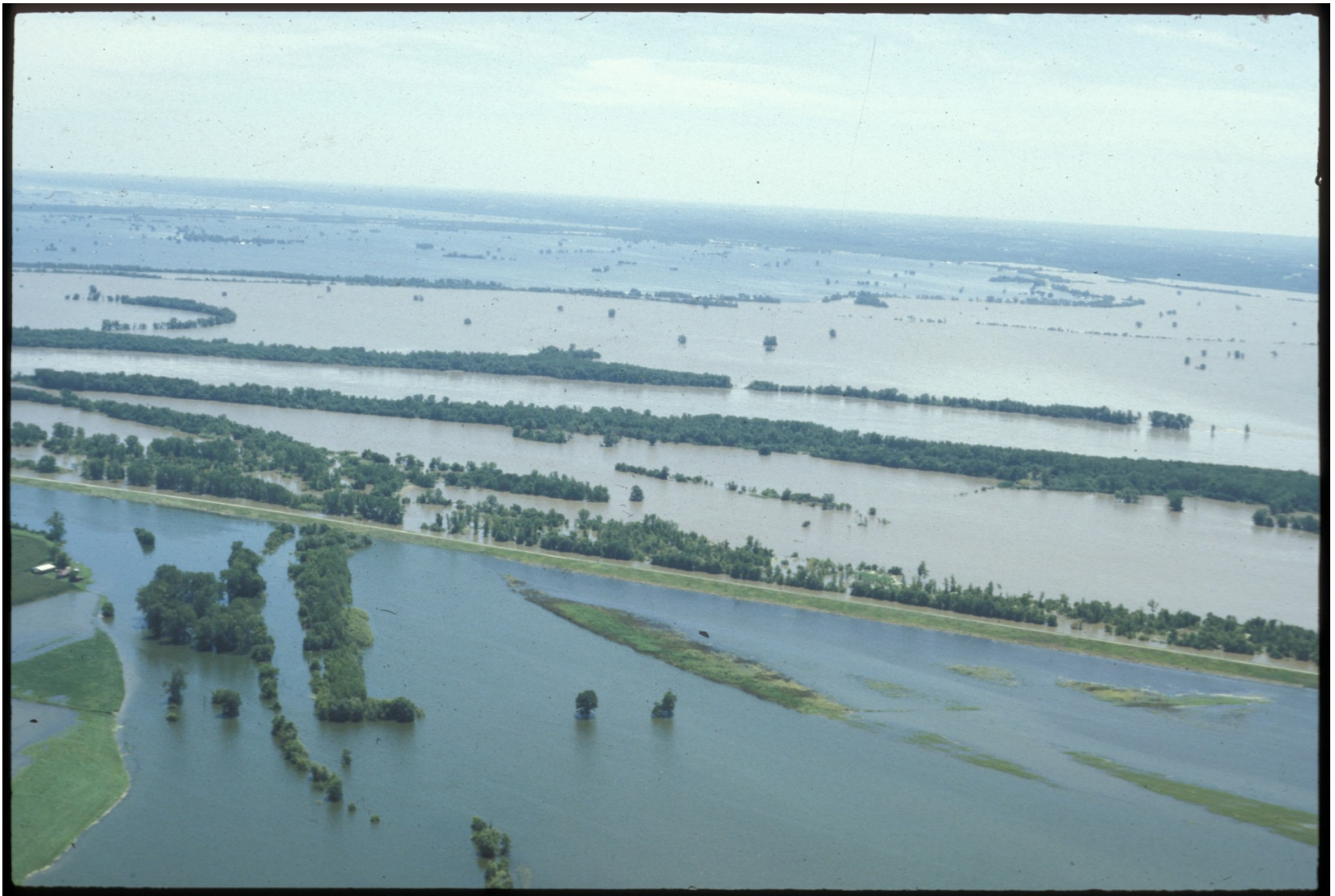
The Mississippi River during the Great Flood of 1993. A levee is visible as a linear feature extending diagonally across the photo.
