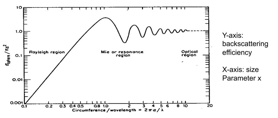
Figure 4.2 Normalized backscattering crosssectional area of a sphere as a function of circumference normalized by radar wavelength  $\lambda$ , a = radius. From Skolnik, 1980, Introduction to Radar Systems, with permission of McGraw-Hill, Inc.
