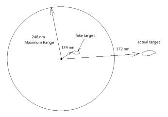
For example, a target at 372 nm away can be displayed at 124 nm range by a radar with  $R_{max} = 248 nm$ .
