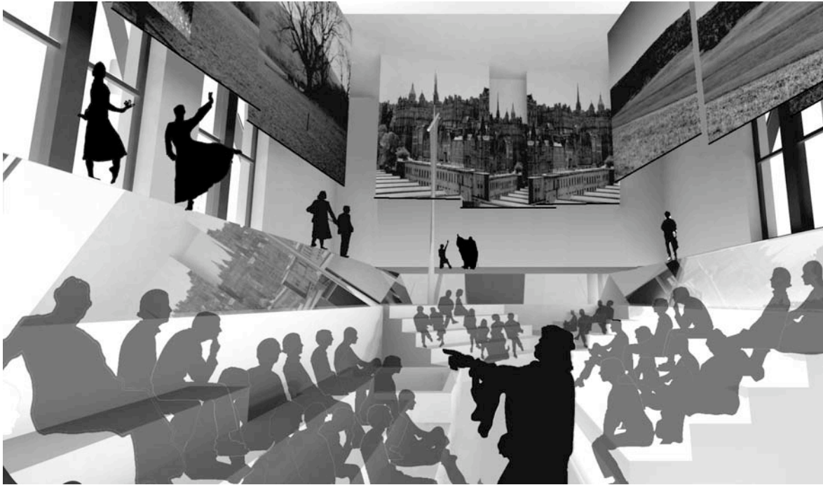
Fig. 1: Interior of Théâtre de l'espace based on Edouard Autant's plan and section. Actors play improvised scenes in lower area between audience bleachers and choreographed drama on upper surrounding stage. Tilted mirrors reflect action behind spectators. (Drawing rendered by Eduardo Luna and author based on sketch by Edouard Autant).
