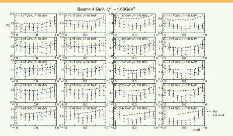
Plane-wave calculation shown here with same normalization as the FSI one (so not fitted)
