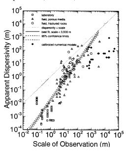
7. The problem in the aquifers of interest is the arrival of toluene at a well field from a leaking gas tank 1000 m away. Give an estimate of the dispersion coefficient based on the scaling relations (Neuman, 1995) shown on the attached graph.
