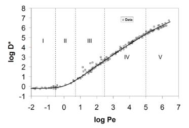
Then compute the Peclet number Pe (= ul/Dm). Using the attached graph (Fried and Combarnous, 1971), find  $D^*$  (=Dd/Dm). Compute Dd (=  $D^*Dm$ ).
