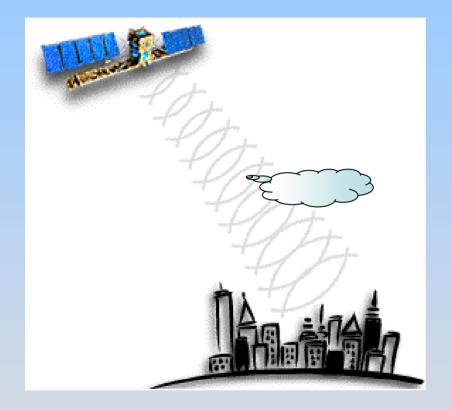
RADAR remote sensing is an `active` imaging technique that utilises the microwave region (~1-100 cm) of the EM spectrum
