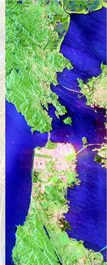
Color composite image red (Pd from T_{22} ) green (Pv from T_{33} ) blue (Ps from T_{11} )
