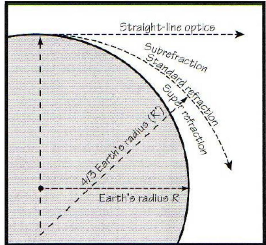
Figure 3.6 Earth's curvature showing the earth (gray circle), earth's radius,  $4/3$  earth's radius, standard refraction, super refraction, subrefraction and straight-line optics. Subrefraction would also be above the straight-line optics line.
