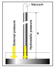
A mercury barometer – an inverted tube of mercury that is sealed at its upper end and stands with its lower end in a bath of mercury. The mercury falls until the pressure it exerts at its base is equal to the atmospheric pressure. By measuring the height of the mercury column we can calculate the atmospheric pressure, provided we can find a relation between height and pressure.
