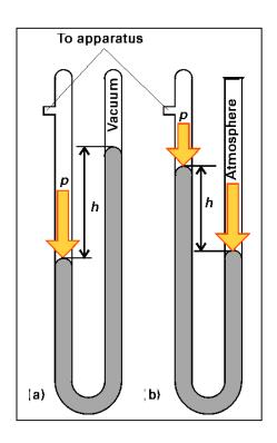
We can measure the pressure of a gas inside a container by using a pressure gauge – the simplest type is a **manometer** – a U-tube containing a liquid. One limb can be connected to the container and the other either sealed (a) or open to the atmosphere (b). The difference in heights of the liquid in the two arms of the open-tube manometer is proportional to the difference in pressure between the gas in the container and the external atmosphere.
