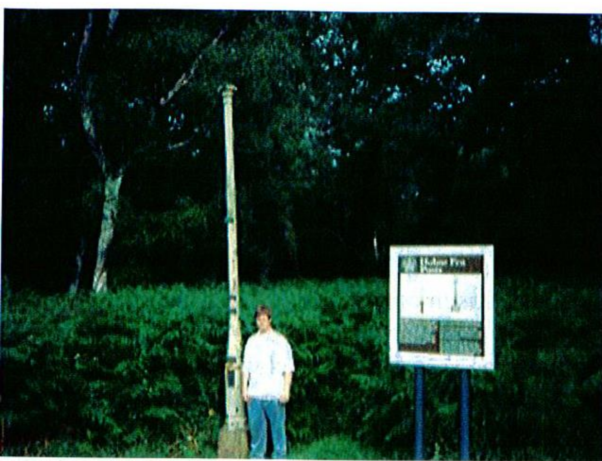
Graduated post sunk in Fens in Holm, England in 1848 with 4.5 m soil subsidence by 1992 (Photo by George H. Snyder, Snyder 2004)
