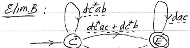
$$\begin{aligned} L(M) &= R_1^* R_2 (R_4 + R_3 R_1^* R_2)^* \\ &= (\underline{dc^*ab})^* (\underline{dc^*ac} + \underline{dc^*b}) [\underline{dac} + (\underline{dab}) \cdot (\underline{dc^*ab})^*, (\underline{dc^*ac} + \underline{dc^*b})]^* \end{aligned}$$
