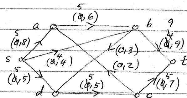
$$\begin{aligned} \text{Val}(f^*) &= \text{net flow into } t \\ &= f^*(\vec{bt}) + f^*(\vec{ct}) = 9 + 5 = 14 \end{aligned}$$
