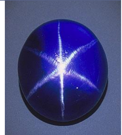
Figure 6.12 Photograph of star sapphire whose long dimension is 8 mm. The star pattern is due to numerous fibrous rutile (TiO 2 ) inclusions parallel to the hexagonally arranged 2-fold rotation axes in the host corundum.
