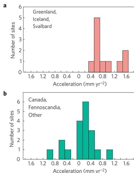
**Figure 3 | Histogram of vertical acceleration for GPS sites. a**, Areas with significant land ice (Greenland, Iceland, Svalbard) with a mean and standard deviation of  $0.87$  and  $0.46 \text{ mm yr}^{-2}$ . **b**, Adjacent North Atlantic areas with only seasonal ice or snow (including northeast Canada and Fennoscandia) with a mean and standard deviation of  $0.04$  and  $0.44 \text{ mm yr}^{-2}$ .
