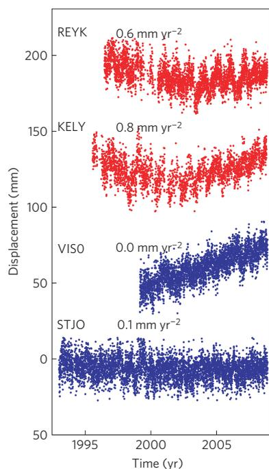
**Figure 2 | Representative GPS time series for the North Atlantic region, showing site name and acceleration.** The red (upper) time series (Greenland, Iceland) show positive acceleration and the blue (lower) time series (Fennoscandia, Canada) show no significant acceleration; for example, VISO shows uplift at an essentially constant rate. All time series are shown in Supplementary Information.
