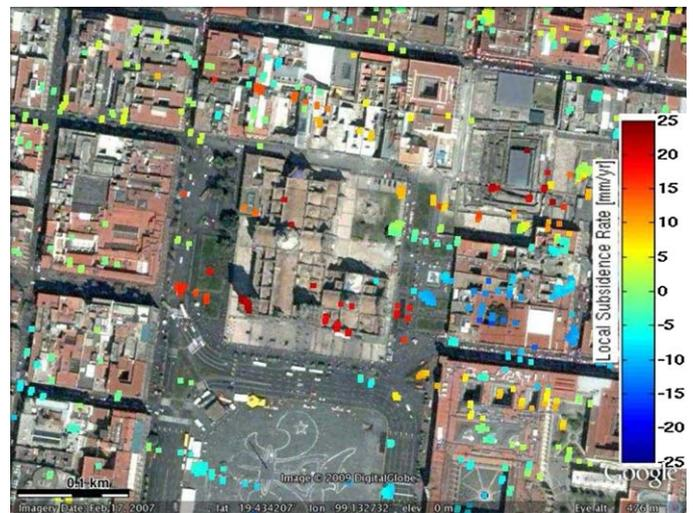
**Fig. 12.** In this figure, red indicates slower than average subsidence rates, and blue indicates faster than average subsidence. Local subsidence measurements around the Metropolitan Cathedral show slower subsidence on the southern part of the building (red circles). (For interpretation of the references to color in this figure legend, the reader is referred to the web version of the article.)
