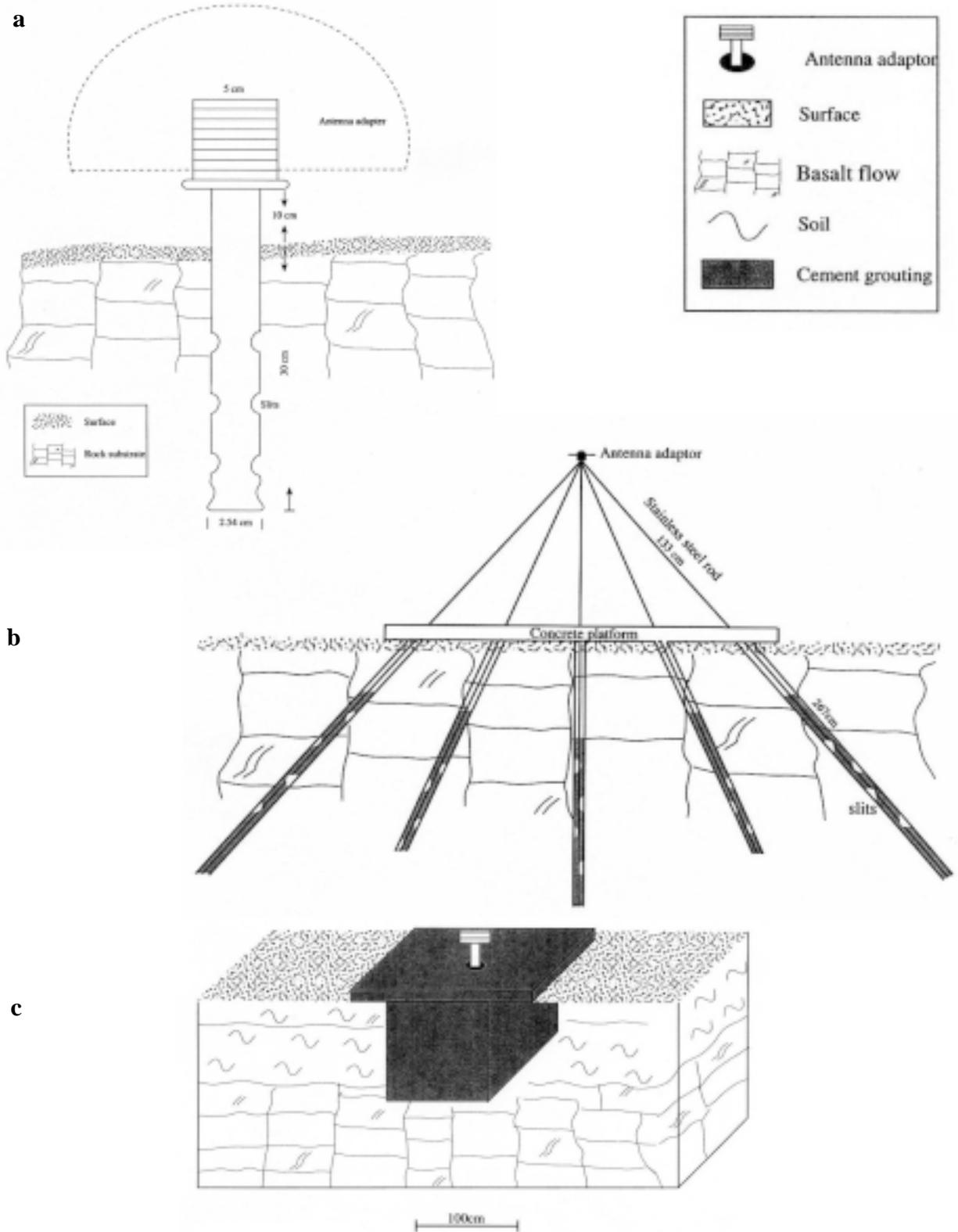
Fig. 2. Geodynamic monument types used in the construction of the GIL network stations: (a) shallow monument, (b) intermediate depth monument, and (c) concrete monument (after Knafo and Wdowski, 2000).
