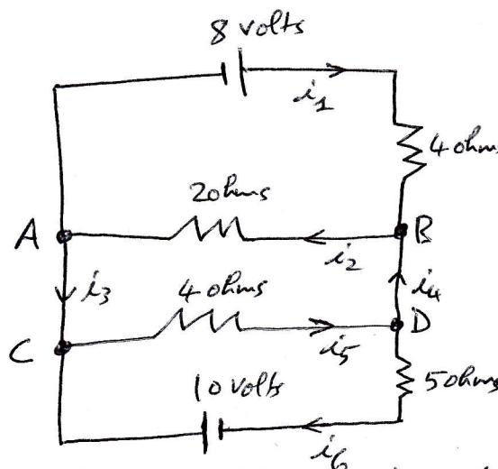
Write down the equations satisfied by the currents  $i_1, i_2, \dots, i_6$ .
